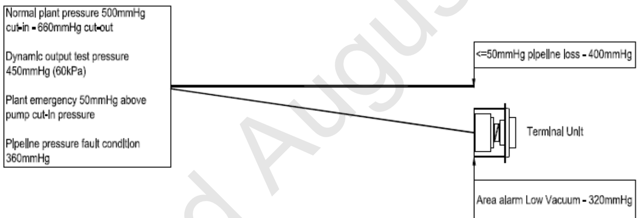
Figure 7: Typical pressures in medical vacuum system under design flow conditions
