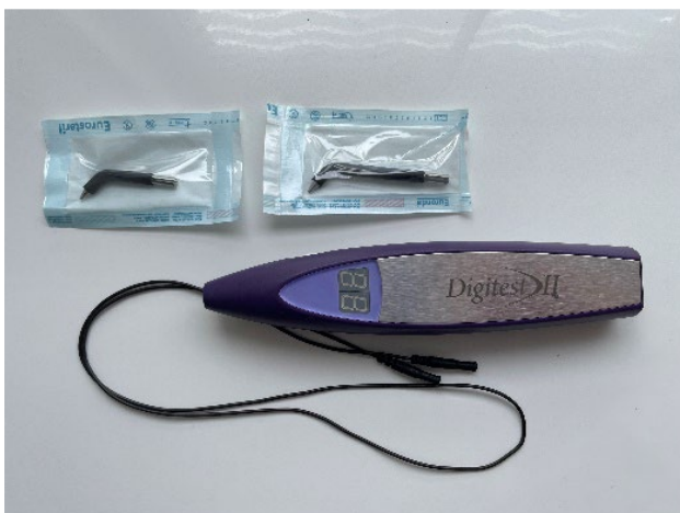
Figure 3.7 - Instrument unsuitable for immersion
