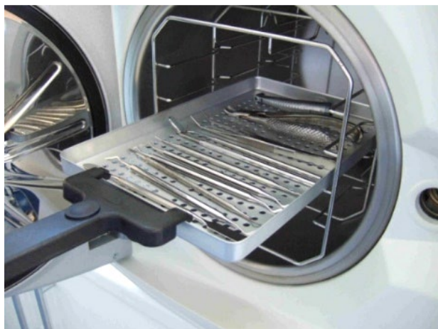
Figure 4.3 - Using a tray lifter to upload instruments
