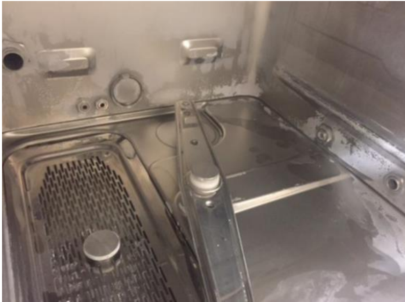
Figure 4.1 - An example of limescale build-up within a WD
