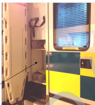
LOW LEVEL Equipment storage cupboard accessed from exterior of ambulance
