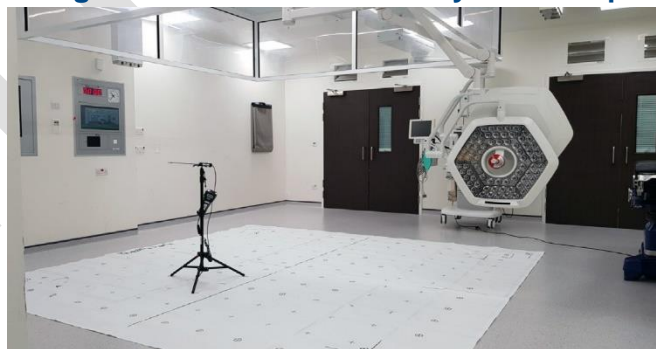
Figure 13: UCV 1m air velocity test set-up
