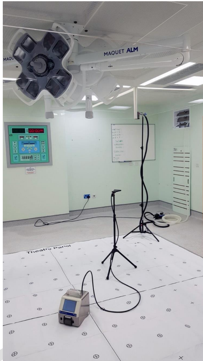
Figure 14 UCV entrainment test setup
