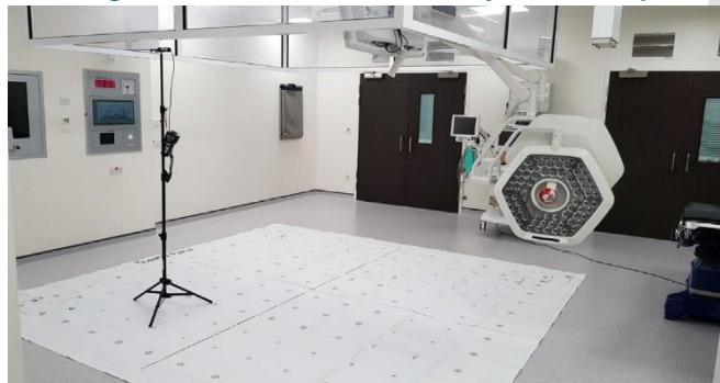
Figure 12: UCV 2m air velocity test set-up
