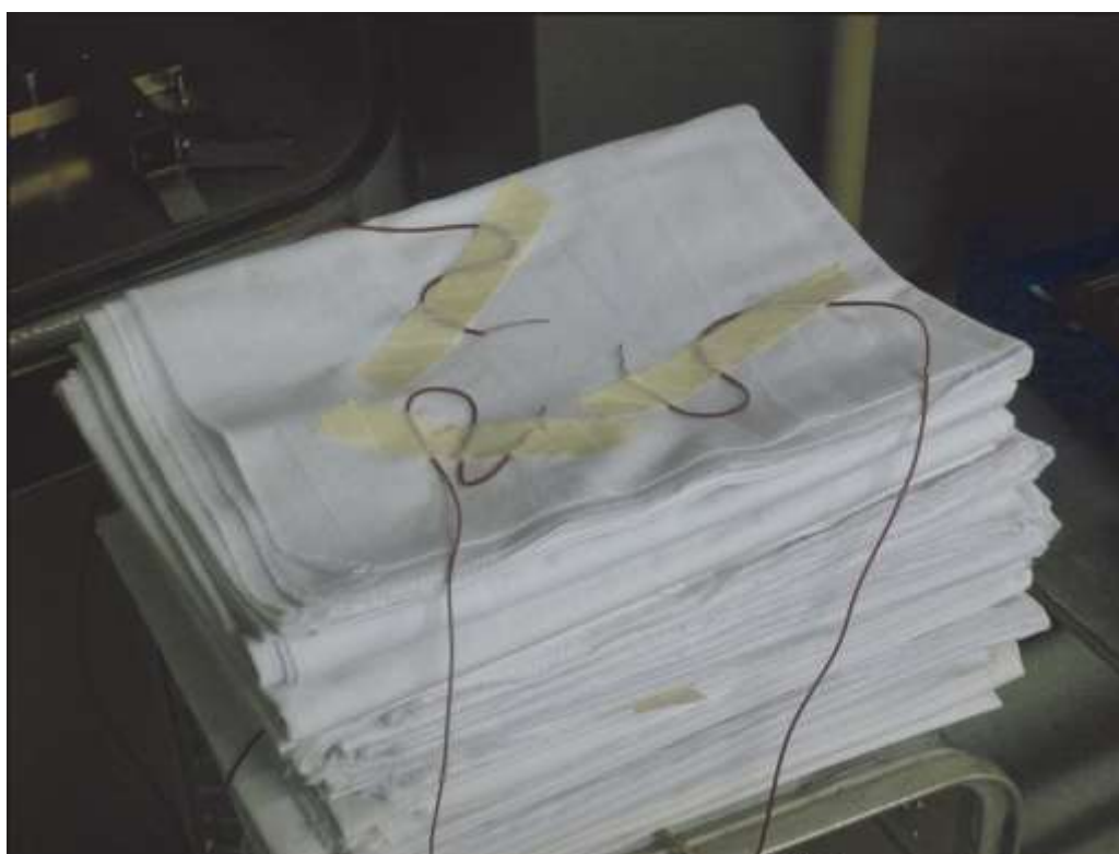
Figure 4: Three sensors in a standard test pack positioned 20 mm below centre, and equally spaced within a diameter of 45 mm
