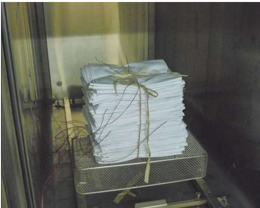
Figure 3: A standard test pack positioned in the chamber on a basket or small tray
