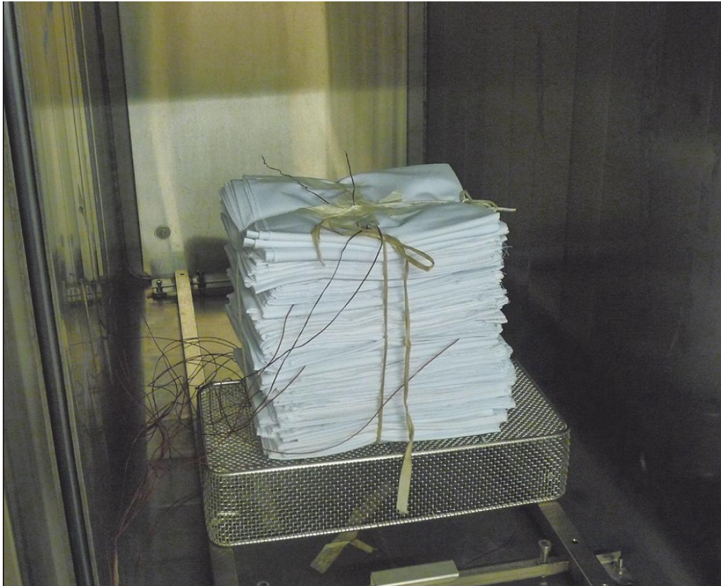
Figure 2: A standard test pack positioned in the chamber on a basket or small tray
