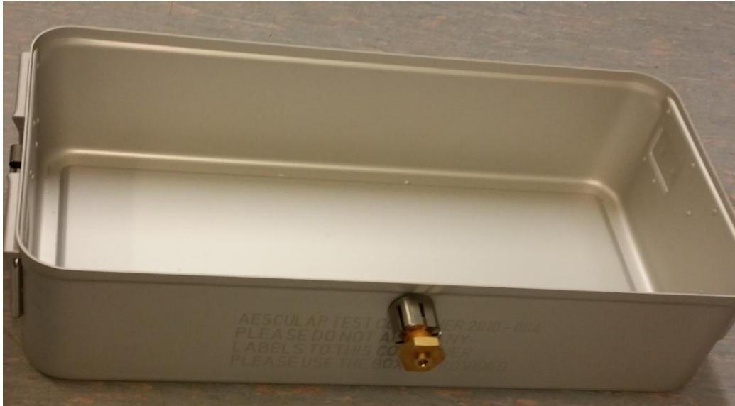
Figure 9: Modified re-useable container with gas-tight thermocouple entry port for thermometric tests
