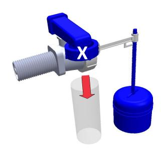
**3.** Once the silencer tube has been removed check that the valve is functioning normally.
