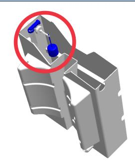
**2a.** Use scissors to remove the transparent plastic silencer tube from the valve, cut as high up as possible (just below the blue retaining ring) and take care not to drop it into the tank. Discard the silencer.
