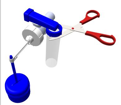
**2b.** Alternatively the silencer can be removed by holding the retaining ring (X) and pulling the tube free. Take care not to drop the tube and retaining ring into the tank. Discard the silencer.
